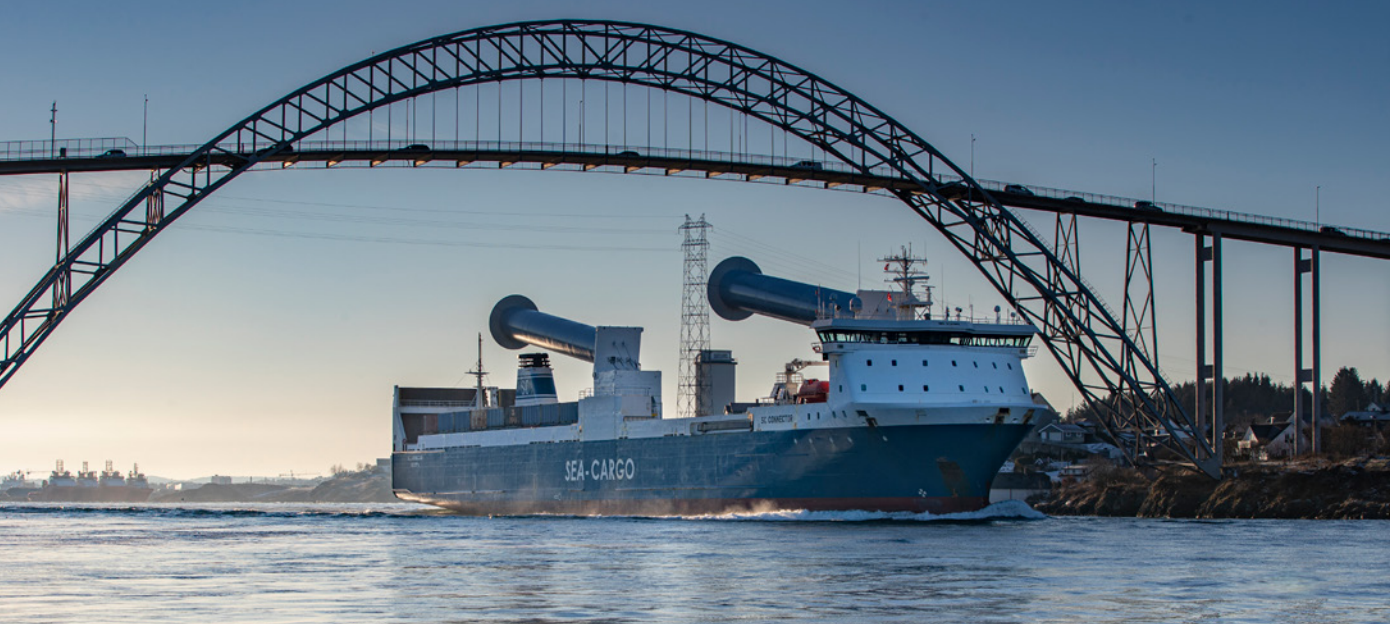
Roro vessel from Sea-Cargo, a new innovation with hybrid technology and two large rotor sails that are estimated to give a 25 % reduction in fuel consumption and CO2 emissions per year. Image: Sea Cargo.
